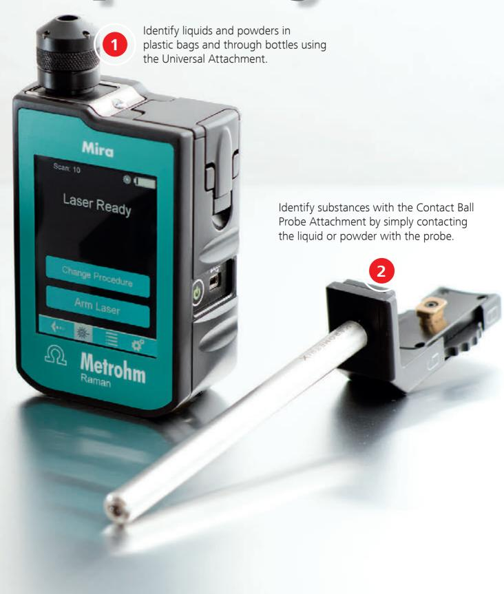
When identifying explosives, you can adjust the laser power of your Mira DS and set a scan delay to allow you to distance yourself from the measurement.
