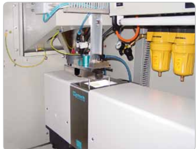
CAMSIZER Online with integrated ionizer to improve sample flow.
