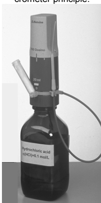
Dosino The buret motor is directly placed onto the reagent bottle. Used for automatic titrators.
