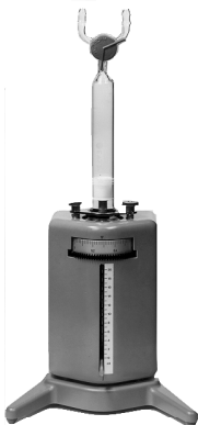
First piston buret (Metrohm 1955) PTFE piston in a calibrated glass tube. Highly accurate volume resolution according to the micrometer principle.
