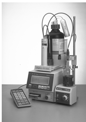
Titrimo Complete automatic titrator. The buret is part of the titrator.
