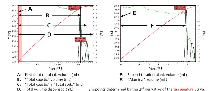
Thermometric titration plots from the determination of total caustic, total soda, and alumina from a sodium aluminate liquor sample.
