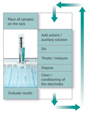
Benefits of an automated analysis using the 898 XYZ Sample Changer: working steps performed by the user in the left column, working steps automated by the 898 in the right.
