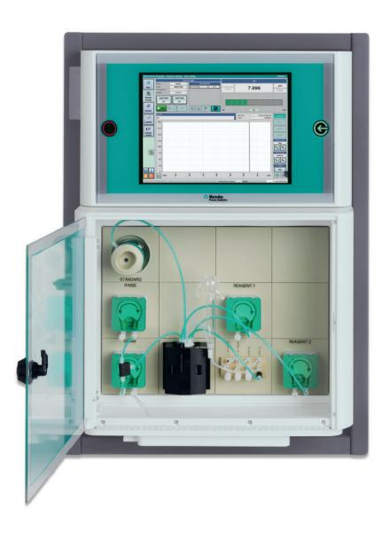
The 2035 Process Analyzer implements fully automated thermometric titration. At the heart of thermometric titration is a fast-responding, highly sensitive temperature sensor. Instead of the electrochemical potential, the endpoint is determined by enthalpy, i.e., the change in temperature in solution during the titration.
