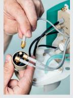
**11. Calibration of measuring inputs** Accurate and reproducible analysis results depend on the detection of minute current and voltage changes. In titration and voltammetry/CVS, specially developed and calibrated tools are used to ensure precision in the testing and **calibration of measuring inputs**.
