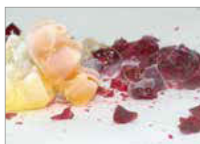
Material embrittled with liquid nitrogen
