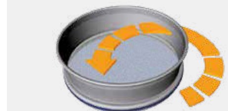
Principle of horizontal sieving
