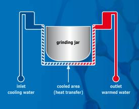
range, i. e. he can set a minimum and a maximum temperature. When the maximum temperature is exceeded, the mill automatically stops and starts again upon reaching the minimum temperature.
